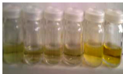
Figure 2. Absorption spectra and color change when dye 1 (0.5 mM) was treated with various analytes (vials from the left: \text{Cl}^- , \text{CH}_3\text{COO}^- , \text{H}_2\text{PO}_4^- , \text{SCN}^- , \text{F}^- and \text{CN}^- as \text{Bu}_4\text{N}^+ salts) in DMSO.
